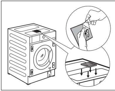
The appliance is also equipped with an adhesive sponge pad **H** that you can find inside the drum. Attach it on the top of the appliance where indicated in the drawing. When levelling the appliance under the furniture, **DO NOT** squeeze the sponge pad.
