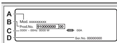
The rating plate reports the model name (A), product number (B), electrical ratings (C) and serial number (D).
