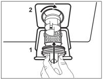
**9.** Put the filter back into the special guides by turning it clockwise. Make sure that you tighten the filter correctly to prevent leakages.
