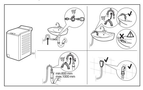
The drain hose should stay at a height of no less than 600 mm and not more than 1000 mm. You can extend the drain hose to maximum 4000 mm. Contact the authorised service centre for the other drain hose and the extension.
