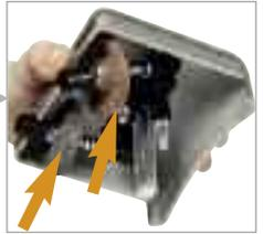
Remove any residue from the sharpening wheels with a brush.
