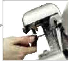
Remove the screw of the blade sharpener.
