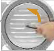
Remove the blade protection screw using the Allen key provided.
