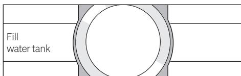
**i** If the action required was carried out, e.g. filling the water tank, the corresponding message and symbol will disappear.
