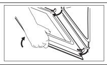
Step 4 Put the door on a soft cloth on a stable surface and release the locking system to remove the internal glass panel.
