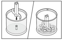
2. Align the Chopper Attachment with the Motor Body and press together. Do not twist the Motor Body into place.
