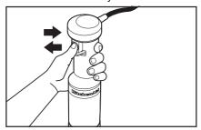
**4.** When chopping is complete, release the Variable Speed Controller.
