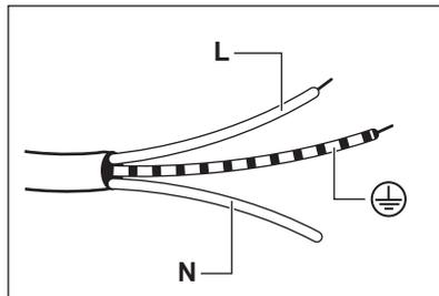
1. Connect the green and yellow (earth) wire to the terminal which is marked with the letter 'E', or the earth symbol
